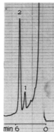
Fig. 6. Separation of 50 \text{ ng} each of formic (1) and acetic acids (2) and 100 \text{ ng} each of propionic (3), isobutyric (4), n -butyric (5), isovaleric (6) and n -valeric acids (7). 15% PPGS on Chromosorb W, argon ionization detector, detector potential 1750 \text{ V} , attenuation \times 1 , argon flow-rate 100 \text{ ml/min} , injection size 1 \mu\text{l} .
